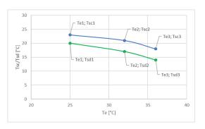
If the unit is controlled according to ambient temperature and its effect on the heating or cooling curve is enabled, the unit changes the water temperature setpoint in either heating or cooling mode at fixed time intervals, based on the difference between the external air temperature measured and the relevant setpoint. The resulting difference is then subtracted from the water temperature setpoint that has been calculated according to the climate curve.
