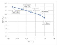
If the unit is controlled according to ambient temperature and its effect on the heating curve is enabled, the unit will change the water temperature setpoint in heating mode at fixed time intervals, based on the difference between the external air temperature measured and the relevant setpoint. The resulting difference is then subtracted from the water temperature setpoint that has been calculated according to the climate curve.
